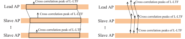
Fig. 6: Extracting the signal frame for one STA at the AP processor via correlating signal streams with L-LTF.
